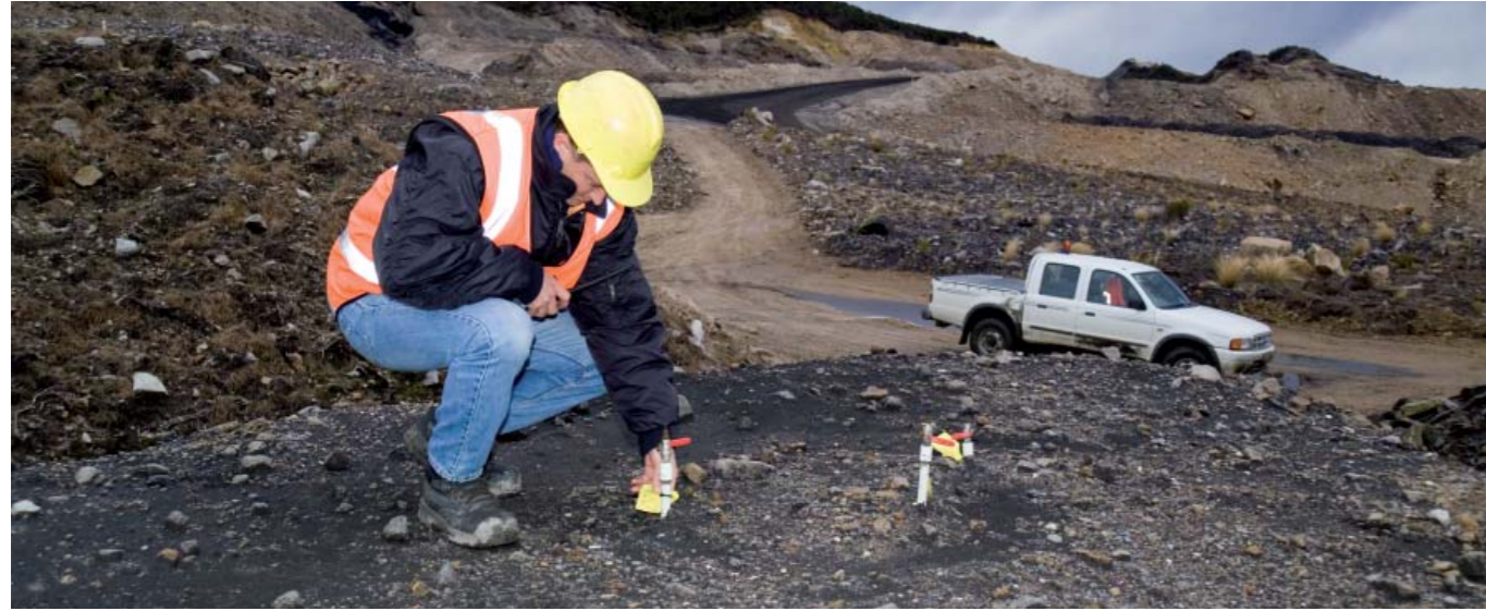
Environmental Operations Manager, Dr Phil Lindsay examines oxygen probes on a fly ash capping trial at Stockton. The alkaline fly ash is being used as a capping material to prevent the penetration of oxygen and water into overburden dumps.
