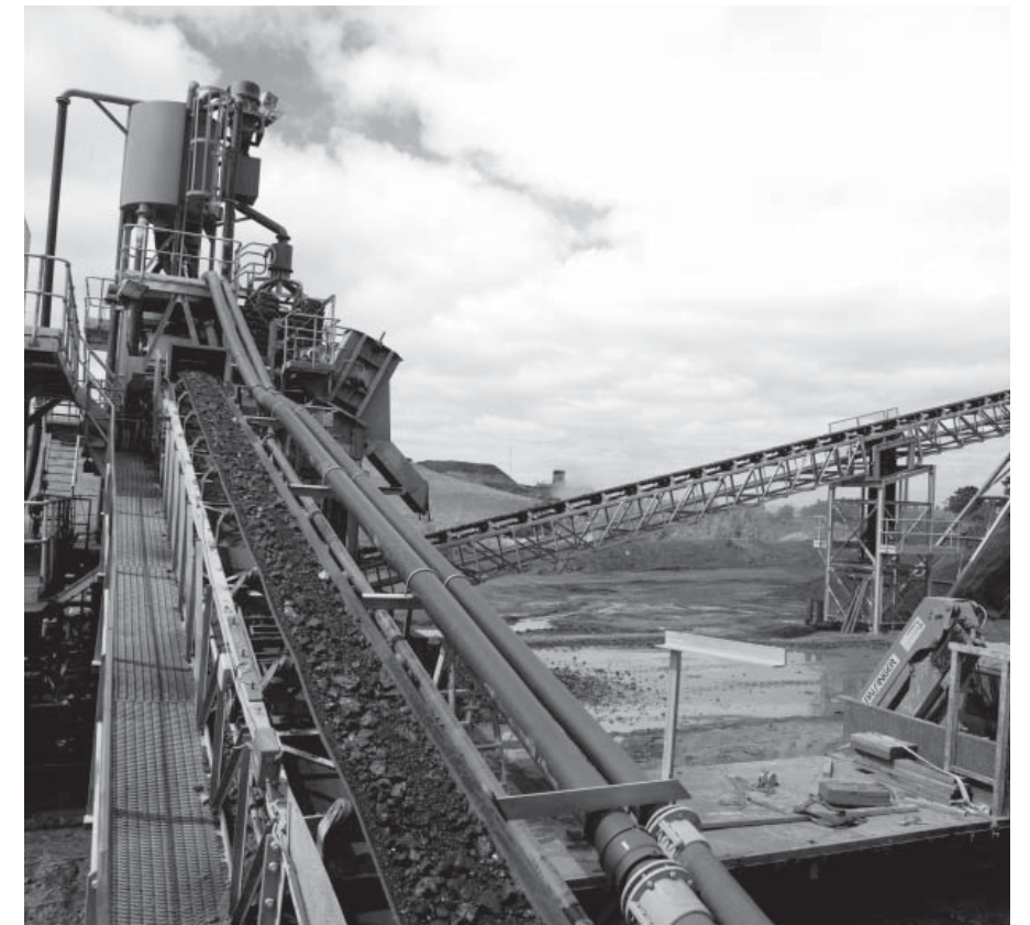
The upgraded washery can process up to 150 tonnes an hour.
